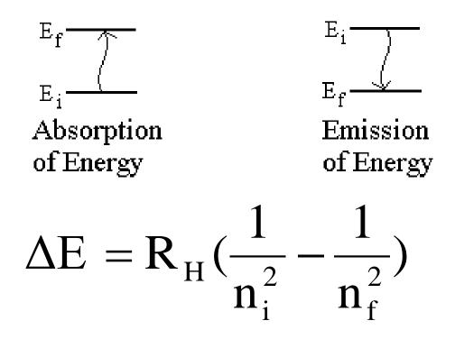
**∆E: energy absorbed or emitted R<sub>H</sub>: Rydberg Constant(2.179×10<sup>-18</sup>J)**  Ex: Calculate the energy absorbed or given off when an electron travels from the n = 5 to the n = 2level.
